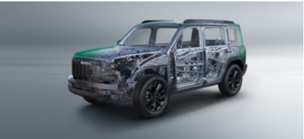
2026 A/E-NCAP Five-Star Rating: reinforced with ultra-strong 2000 MPa steel in key body areas.
